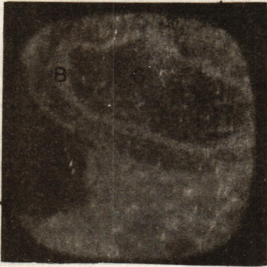
Fig. 5 Sample No. 3 shows Oolites with Goethite (G) in the centre and Boehmite (B) in the outer rim, Clay minerals are seen in the darker part. (Pol. X4).
