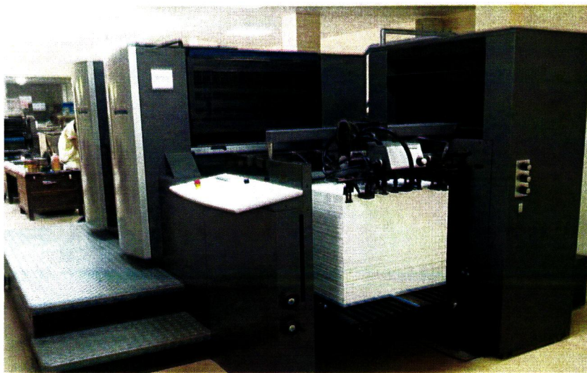
Heavy Duty Printing Machine Heidelberg Speedmaster SM 74-2
